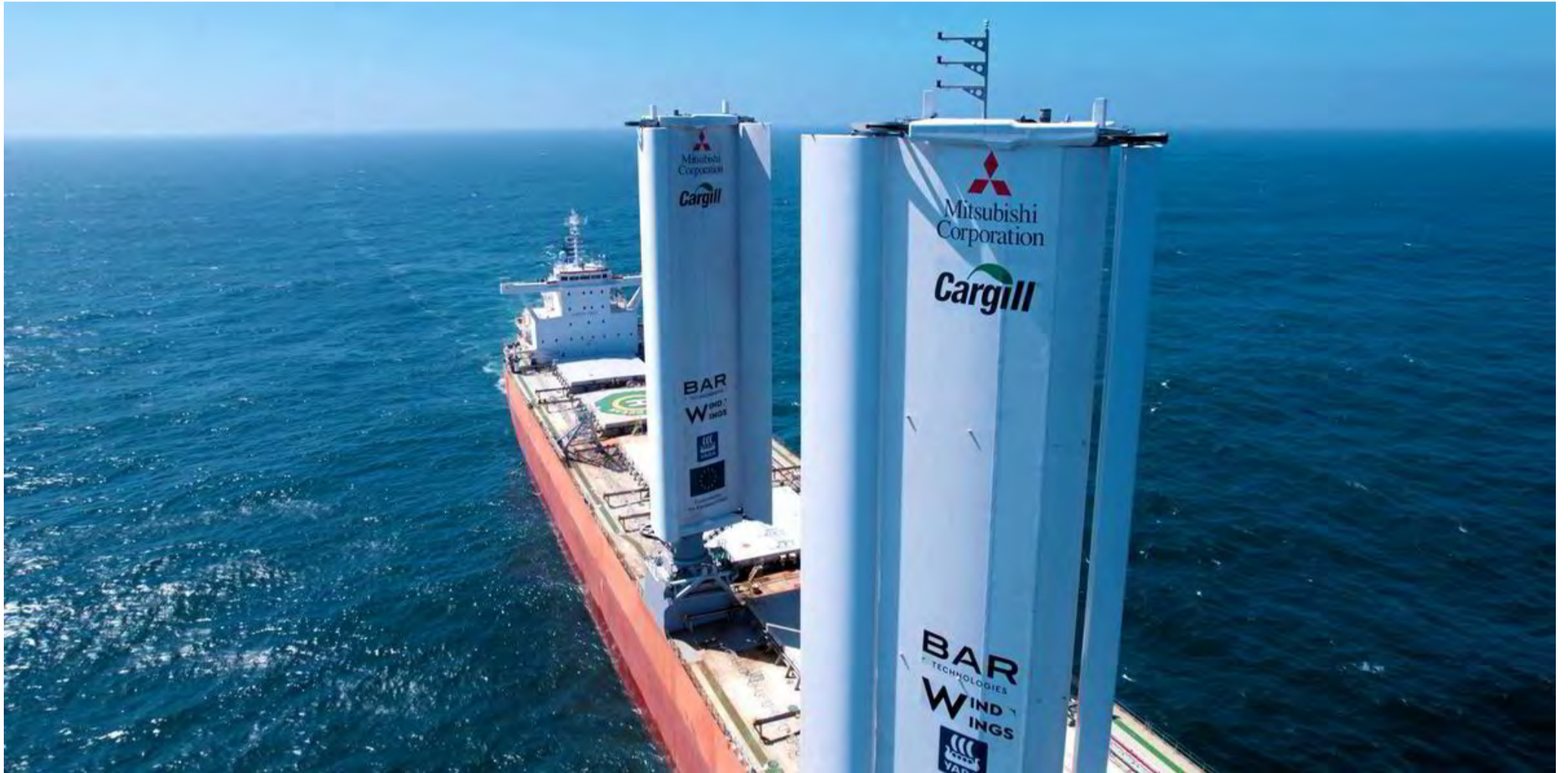
Two WindWings sails tower over Mitsubishi Corp's Pyxis Ocean. The ship is chartered to Cargill Ocean Transportation. Photo: Cargill
