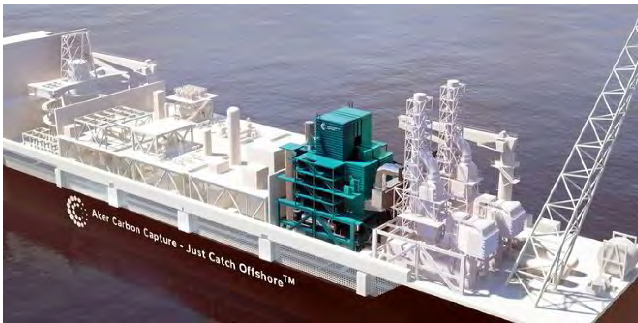
A rendering of Aker Carbon Capture's modular technology Just Catch Offshore CCS system. Photo: Aker Carbon Capture
