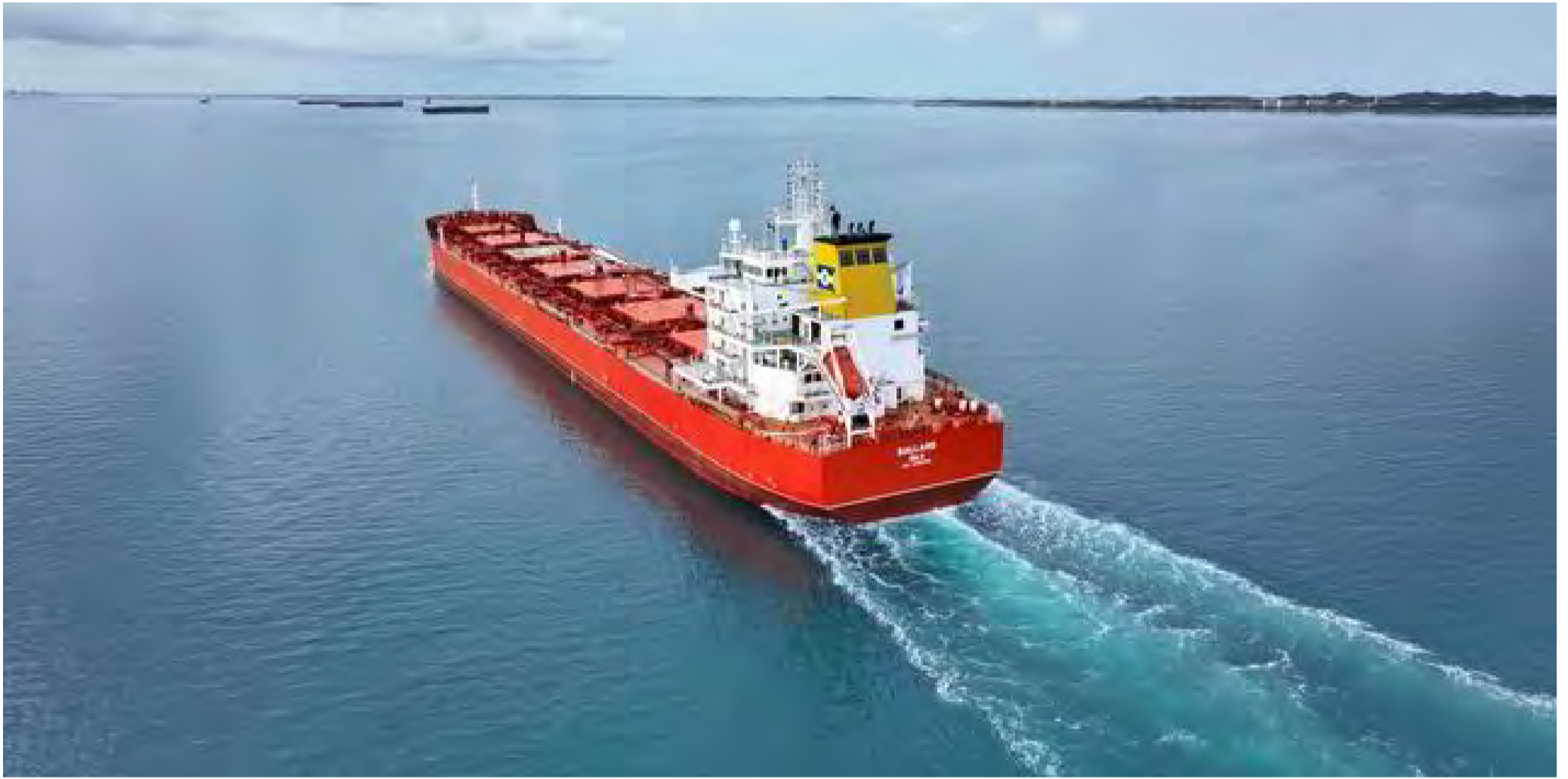
KCC's Ballard with Silverstream bubbles from its air lubrication system. Photo: KCC
