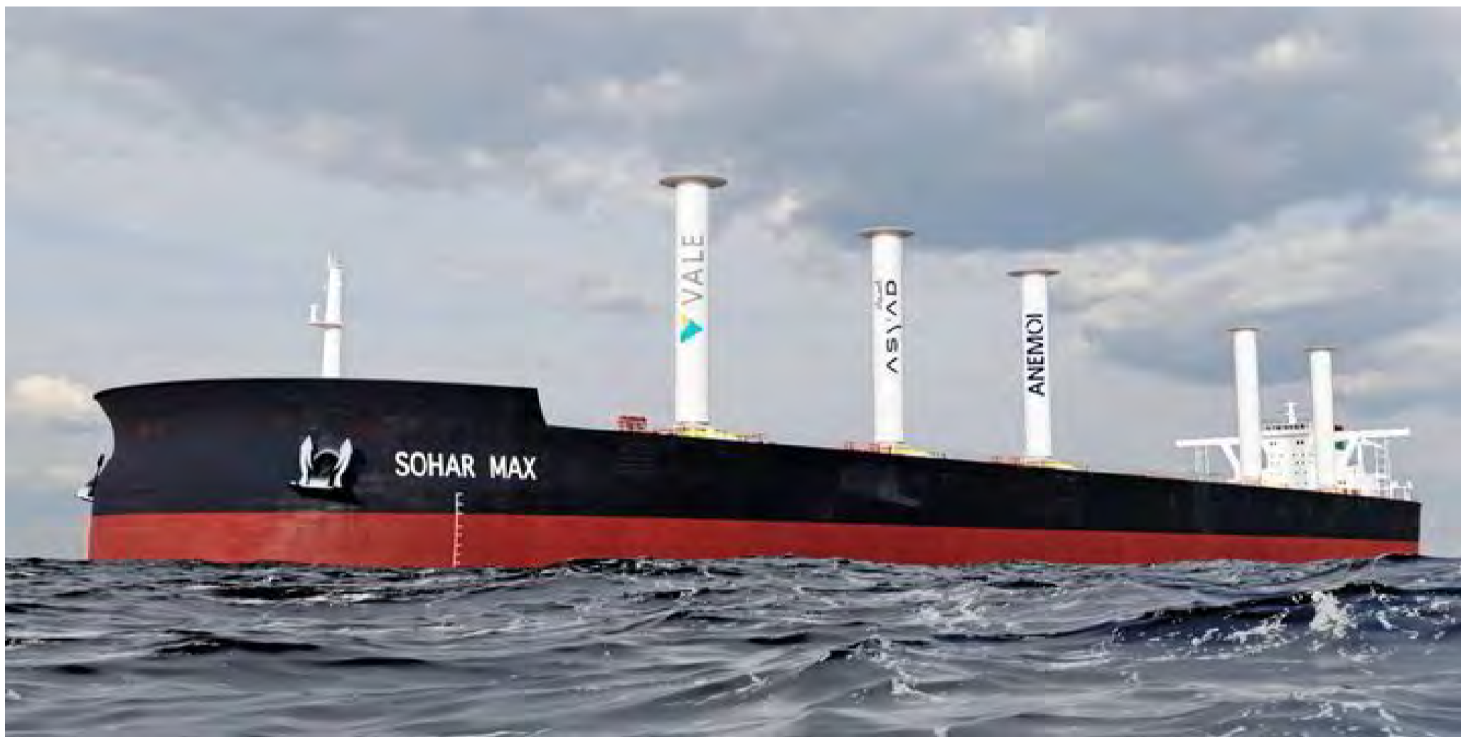
How Vale's Sohar Max will look with Anemoi rotor sails. Photo: Vale
